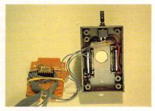
Photo 3. Power supply installed and wired to camera chip board.
